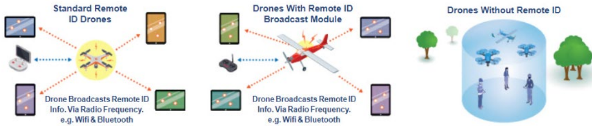
Figure 61: Three ways of complying with Part 89 Remote ID rules. Standard RID is the only option for operating Beyond Visual Line of Sight. Source: FAA UAS Remote Identification. https://www.faa.gov/uas/getting_started/remote_id
