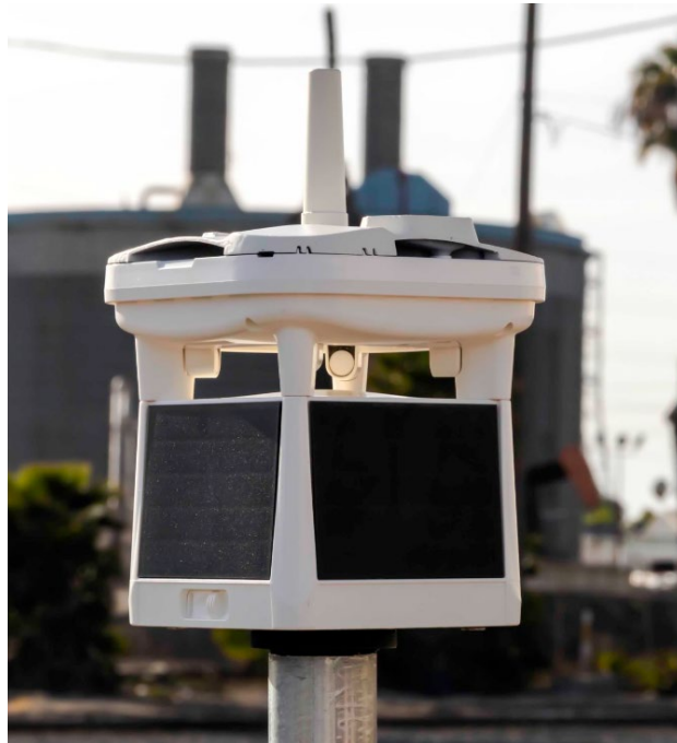
Figure 52: Example of a micro weather sensing unit that combines multiple weather sensors into a single package. Source: Intellisense Systems https://www.intellisenseinc.com/products/weather-stations/mws-c400/
