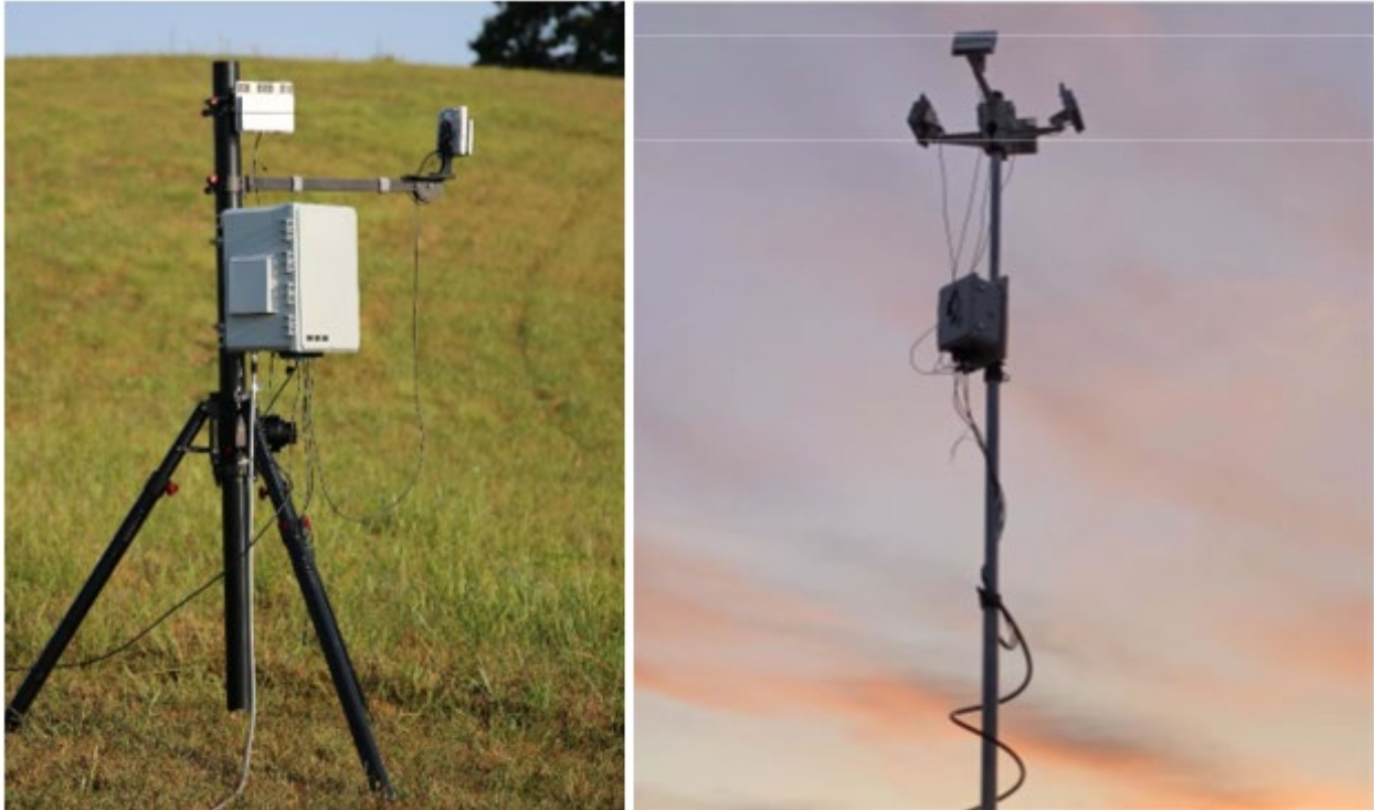
Figure 41: A two-panel Echodyne Echoguard array with connection hub shown as a ground-based sensor mounted on a tripod (left), as well as a four-panel array mounted on a mast for increased viewshed (right). Source: Virginia Tech Mid-Atlantic Aviation Partnership. https://maap.ictas.vt.edu/
