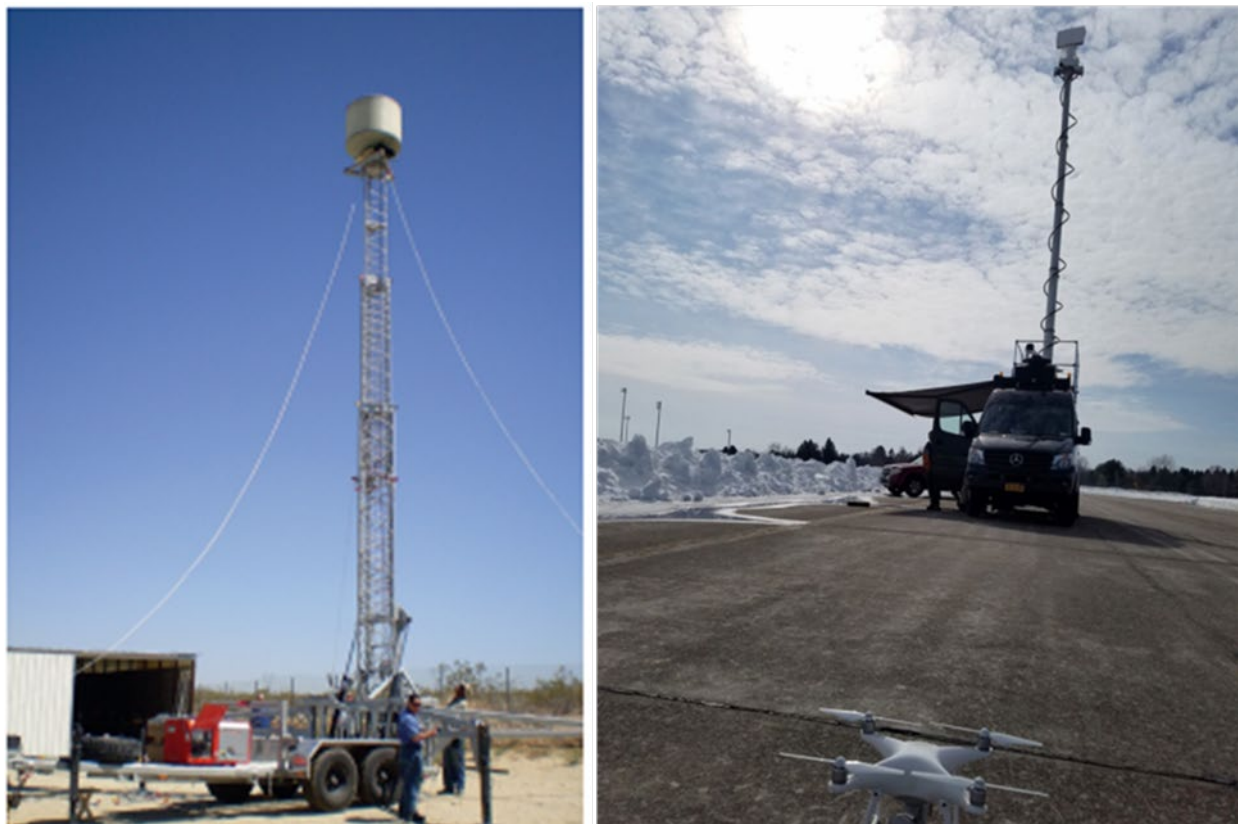
Figure 16: Airspace surveillance infrastructure used in the New York BVLOS corridor. An SRC LSTAR (V)2 radar (left) and a mobile operations command center (right). Source: SRC https://www.srcinc.com/pdf/Radars-and-Sensors-LSTAR-V2.pdf , NUAIR https://nuair.org/photos/
