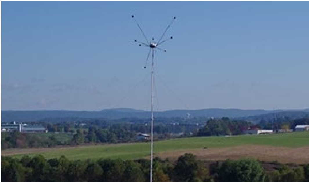
Figure 47: SARA TASA acoustic node deployed on a telescoping mast. Source: Virginia Tech Mid-Atlantic Aviation Partnership. https://maap.ictas.vt.edu/
